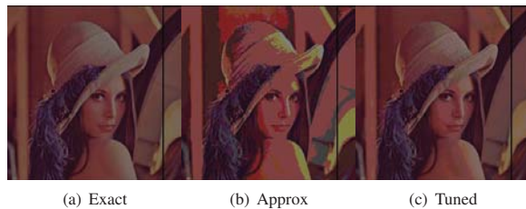
Figure 9: Output quality comparison for Blur application running on (a) exact computing, (b) approximate mode ( PSNR = 25dB ) and (c) tuned computing with PSNR = 34dB and 13% run on precise CFPU.
